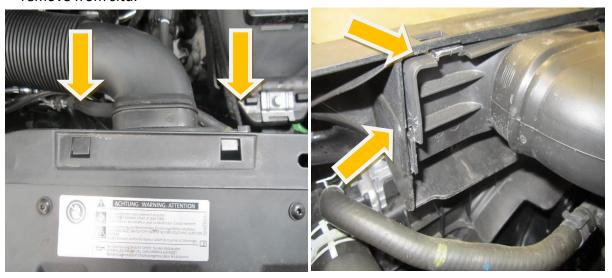
**5**. Pull the airbox sharply in an upwards motion to remove.
