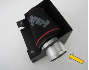
8. Fit the cold air tray into position then using a 5mm Allen Key tighten the mounting bracket into position.
