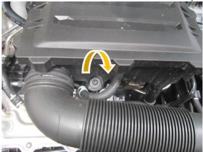
3. Locate the hose clamp at the rear of the airbox and remove.
