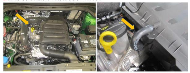
2. Using a T30 torx drive remove the torx fastener that holds the airbox in position.
