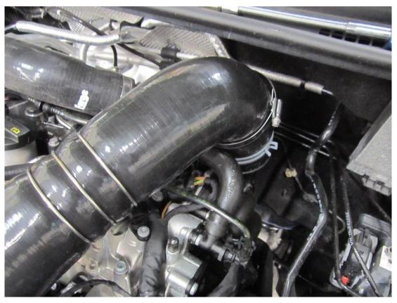
**10**. Attach the opposite end of the silicon hose to the filter along with the crankcase breather.
