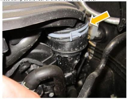
**4.** Using a flat bladed screw driver pry open the tabs that hold the air scoop in position and remove from situ.
