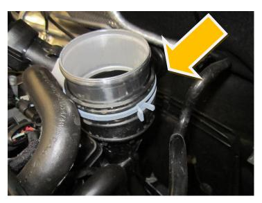
7. Place the forge high flow air filter into the intake tray then insert the alloy coupler into the high flow air filter.
