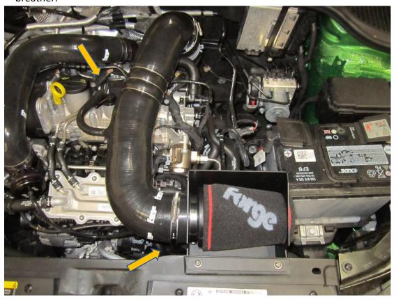
**11.**Tighten the hose clamps with a 7mm socket drive or flat bladed screwdriver and check that all fixings are secure.
